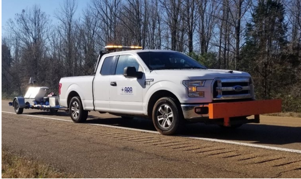
Figure 2. ARA's Falling Weight Deflectometer
